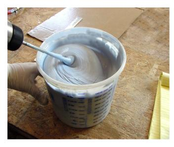
Mix for another 2 minutes under low speed and then allow the air bubbles to rise to the surface for about 10 minutes. Using the spatula gently stir out the surfaced air bubbles. Transferring the mixed material from the mixing container to another container will guarantee a homogenized and a uniformly mixed resin batch.
