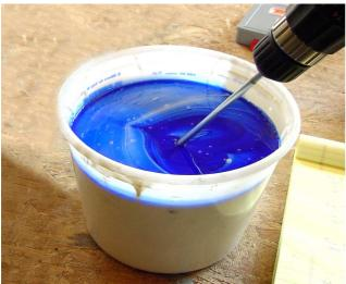
Attach a mixing blade to hand drill and mix at a low speed. Avoid mixing the Silicone too aggressively to avoid excess air entrapment. If available, degas the resin mixture using a vacuum technique to remove any entrapped air bubbles. Since the MAX RTV 662 has a four-hour working time, most of the air bubbles will release by it self. Mix until a uniform color is achieved and no color streaks are visible.
