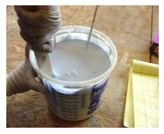
Transfer the entire mix into another container and continue mixing while making sure to scrape the sides and the bottom of the container with a spatula to insure that all the material is well incorporated.
