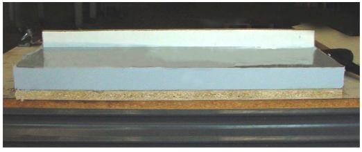
Carefully remove the end plates by gently tapping it with a rubber mallet. Cut away any flash material by running a razor blade or a pair of scissors level to the mold surface. Carefully pry off the side plates. In a corner of the mold gently peel back the Silicone mold upwards and away from the base plate. Use a flat blade screwdriver or plastic spatula to help pry the mold free.
