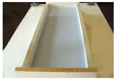
Allow the mold to cure undisturbed for at least 24 hours. Longer curing time may be necessary when curing below 70°F. After 24 hours, check the surface hardness of the mold. It should feel firm and tack free. If a Shore A Durometer Hardness tester is available, check the hardness, a 57 to 62 reading will indicate that it is ready for demolding.
