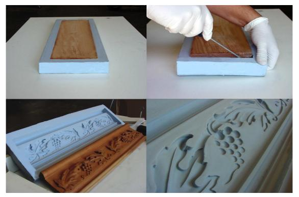
The whole mold should peel away from the base plate revealing the backside of the master part. Cut away or trim off any flash material that might have seeped in between the master part and the base plate. If the master part was properly sealed to the base plate, the mold should be level with the master part.
