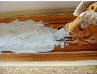
Now we are ready to apply the mixed Silicone resin to mold box. Since our master part is very detailed, we want to make sure that we capture all of the details without any defects caused by pockets of air bubble. An effective way of doing this is by pre-coating the master part with a layer of Silicone resin with a brush. Brushapply the Silicone resin liberally directly on the design of the master part. Use the brush tip to aide the resin into the crevices, nooks and crannies.
