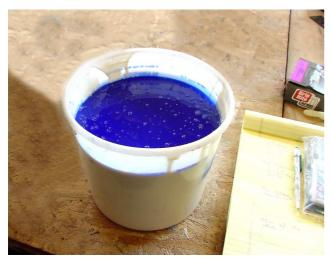
In a clean container weight out the correct amounts of resin and catalyst, typically mixing with a spatula or a mixing stick is recommended. Because of the volume of resin we will be using for this project, we will be utilizing a low speed mixer.
