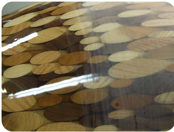
MAX 1618 A/B polished using fine grit sandpaper.
