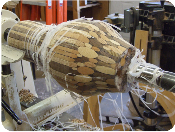
MAX 1618 A/B can be machined after full cure.
