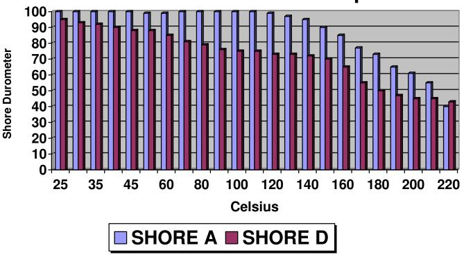
A 6 inch by 6 inch by ¼ inch cured sample of the MAX HTE was exposed to ascending temperature condition and the surface hardness was tested using a both Type A and Type D Shore Hardness Durometer. Shore Hardness determines the resistance of a plastic substrates' resistance to surface deformation from a constant load.
