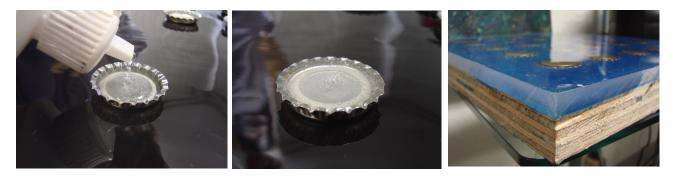
The bottle caps were filled with MAX CLR to eliminate the cavity. It is then bonded to the base substrate to prevent it from moving during the imbedding process.
